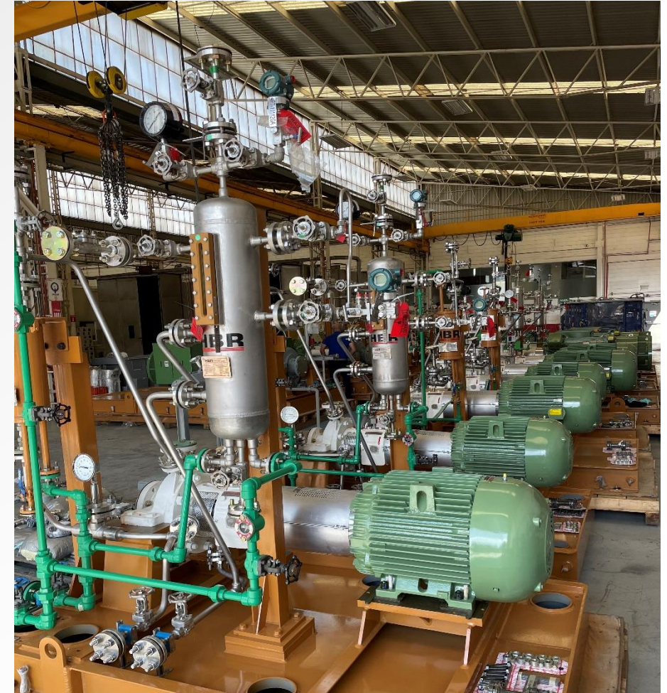
Pump skids in our Santa Clara, Mexico facility awaiting sensors for completion
