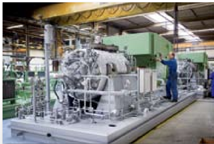
Barrel pump to be used in LNG Pipeline service.
