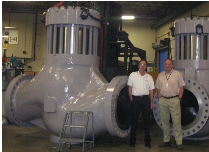
36" Control Valves for Crude Oil Pipeline
